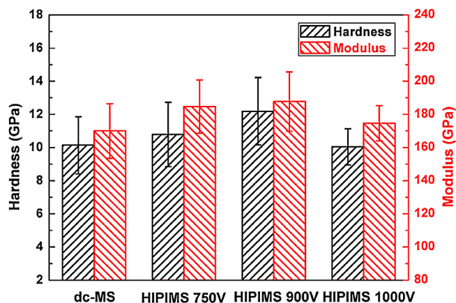
Fig. 5. Hardness and elastic modulus of the GLC films deposited at different conditions.
