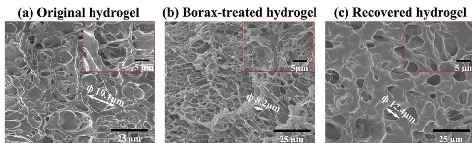
Figure 6. SEM images of the original PAAm/PVA hydrogel (Sample C), as well as samples treated in aqueous 0.08 M \text{Na}_2\text{B}_4\text{O}_7 solution for 5 min and retreated in \text{Na}_2\text{HPO}_4 -citrate buffer solutions (pH = 2.2) for 7 min.
