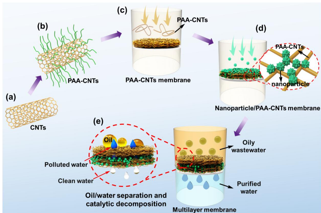
Scheme 1. Fabrication of multi-functional CNTs composite separation membrane by filtration. (a, b) PAA modified CNTs (PAA-CNTs). (c) PAA-CNTs membrane prepared by vacuum filtration. (d) The deposition of catalytic nanoparticles in PAA-CNTs membrane. (e) The resultant multilayer PAA-CNTs/Pd@Pt/PAA-CNTs composite membrane is employed for oil/water separation and catalytic decomposition.
